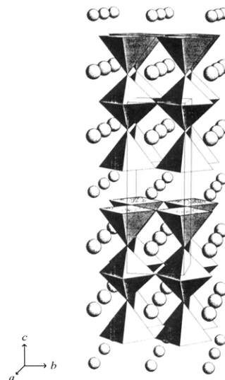
Figure 12. Idealized structure of \text{LaBa}_2\text{Cu}_2\text{TaO}_8 after Rey et al. 30 The octahedra are \text{TaO}_6 and the square pyramids are \text{CuO}_5 . The smaller spheres are lanthanum and the larger are barium.
